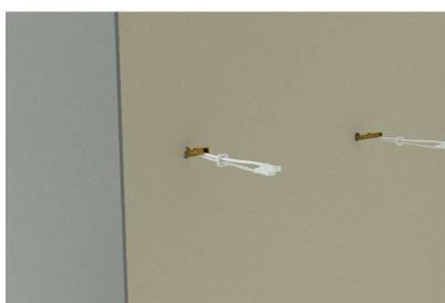
**Step 4**Insert ¼" toggle type wall anchors in locations as marked
