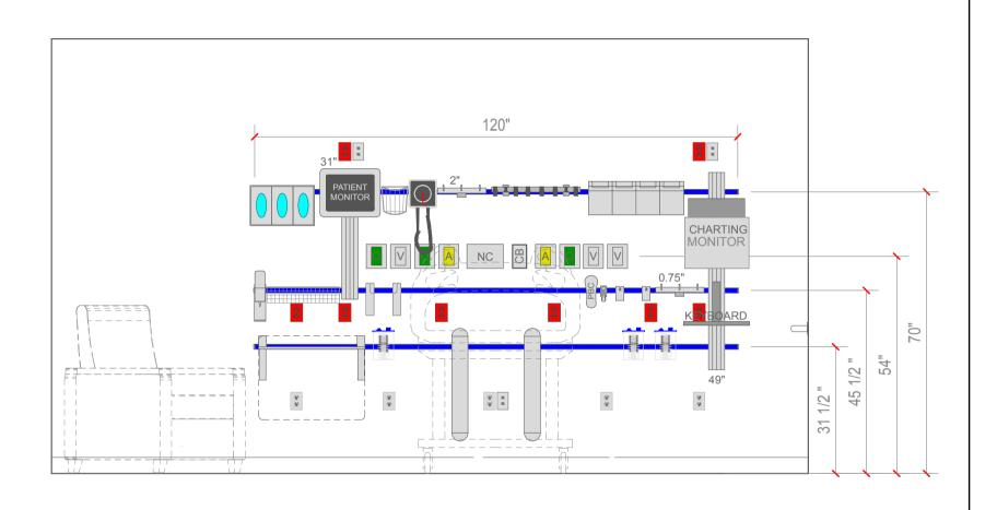
PALADIN HEALTHCARE PROVIDES ONLY THE GCX CHANNELS FOR OWNER SUPPLIED PATIENT MONITORS, COMPUTER EQUIPMENT, AND THE MOUNTS THAT ATTACH THOSE ITEMS TO THE GCX CHANNEL.
