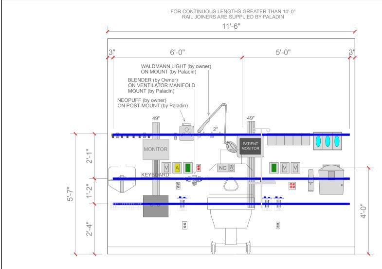
PALADIN HEALTHCARE PROVIDES ONLY THE GCX CHANNELS FOR OWNER SUPPLIED PATIENT MONITORS, COMPUTER EQUIPMENT, AND THE MOUNTS THAT ATTACH THOSE ITEMS TO THE GCX CHANNEL.
