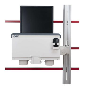
GCX Channel to span (3) rails at 10-20" between rails, but no more than 35" maximum and 25" minimum total between top and bottom rail.
